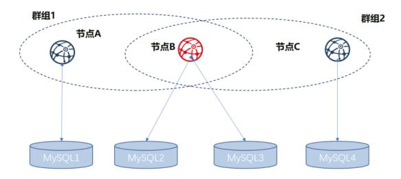
As shown in the above figure, NodeB belongs to multiple groups. The database instances which are corresponded by the same node in different groups are separate. For distinguishing the same node in different groups, the nodes of A, B, and C are respectively represented with Group1\_A (NodeA in Group1, same as below), Group1\_B, Group2\_B, and Group2\_C.
